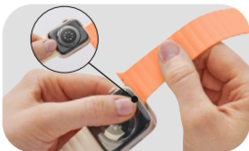
To remove the strap, press the button and push it out.
