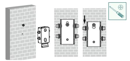
• First hang the wall bracket on the top screw, as shown.
