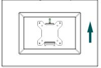
When mounting the VESA plate onto the back of your TV set, ensure that the fastening screw is at the top.
