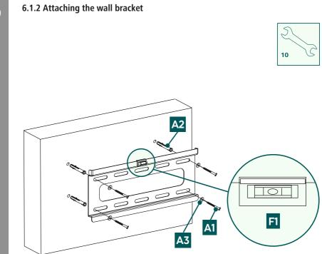
• Attach the wall bracket to the wall as shown above using the enclosed mounting material ([A2] plug, [A3] M6 washer, [A1] 6x70 mm screw and the [F1] spirit level).
