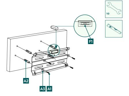
• Attach the wall bracket to the wall as shown above using the enclosed mounting material ([A2] plug, [A3] M6 washer, [A1] 6x50 mm screw and the [F1] spirit level).
