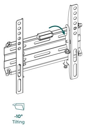
• To adjust the tilt angle, open the fastening screws at the side, set the required tilt, and then secure the screws in place again.
