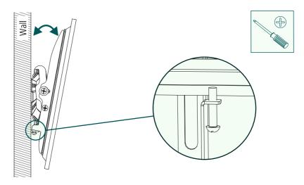
• Then attach the fastening screws on both supporting arms, as shown above.
