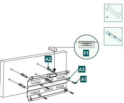
• Attach the wall bracket to the wall as shown above using the enclosed mounting material ([A2] plug, [A3] M6 washer, [A1] 6x50 mm screw and the [F1] spirit level).
