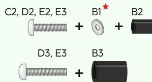
$$\text{M8x50} + \text{Ø}8x5 = \text{M8x45 (D4)}$$
