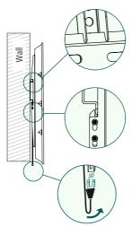
• The ends of the securing cords can be fastened at the back to the wall bracket using the magnets.
