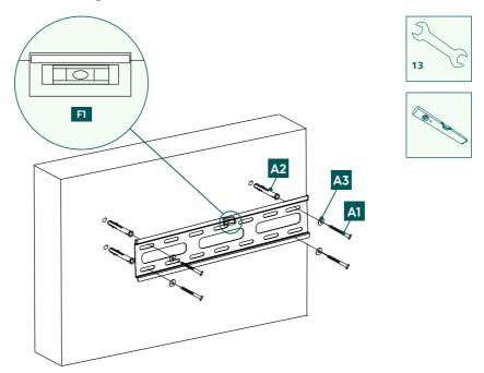
• Attach the wall bracket to the wall as shown above using the enclosed mounting material ([A2] plug, [A3] M8 washer, [A1] 8x50 mm screw and the [F1] spirit level).
