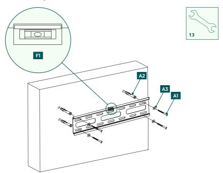
• Attach the wall bracket to the wall as shown above using the enclosed mounting material ([A2] plug, [A3] M8 washer, [A1] 8x50 mm screw and [F1] spirit level).
