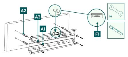
• Attach the wall bracket to the wall as shown above using the enclosed mounting material ([A2] plug, [A3] M6 washer, [A1] 6x50 mm screw and the [F1] spirit level).
