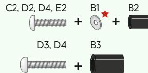
$$\text{Bolt} + \text{Flat Washer} = \text{Distance Element}$$
