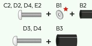
$$\text{M8x50} + \text{Ø 8x5} = \text{M8x45 (D4)}$$
