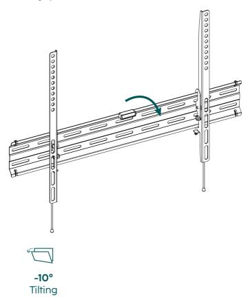
Open the side fastening screws, set the desired tilt and tighten the screws again.
