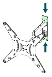
• Then attach the two enclosed covers to the bracket.
