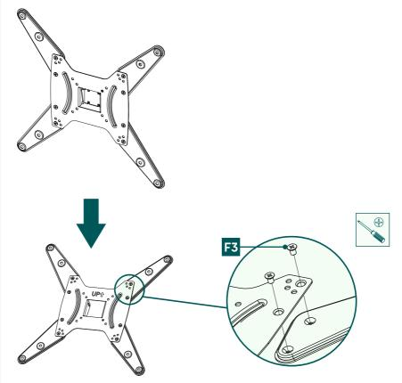
Mount the supplied adapter plates on the back of the VESA plate using screws [F3].
