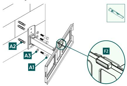
• Attach the wall bracket to the wall as shown above using the enclosed mounting material ([A2] plug, [A3] M6 washer, [A1] 6x70 mm screw and the [F2] spirit level).
