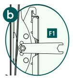
• Then fix the lateral fastening screws using the hexagon ring spanner [F1]).
