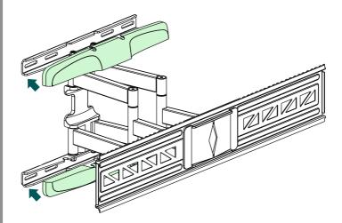
• Then attach the two enclosed covers to the bracket.
