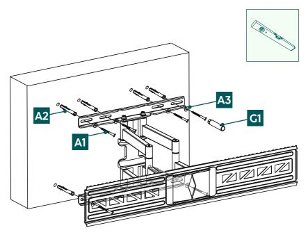
• Attach the wall bracket to the wall as shown above using the enclosed mounting material ([A2] plug, [A3] M8 washer, [A1] 8x60 mm screw, [G1] pipe socket spanner and [F2] spirit level).
