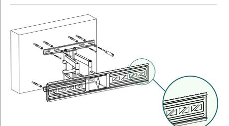
Before installation, ensure that the grooved side of the VESA plate is pointing upwards.
