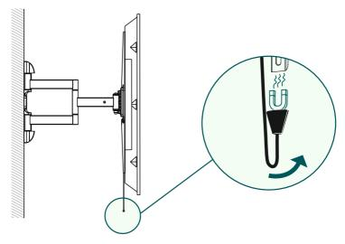
• The ends of the securing cords can be fastened at the back to the wall bracket using the magnets.
