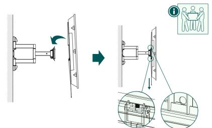
• Pull the securing cord downwards and hang the TV set with the mounted VESA arms on the wall bracket as shown above until it audibly engages.
