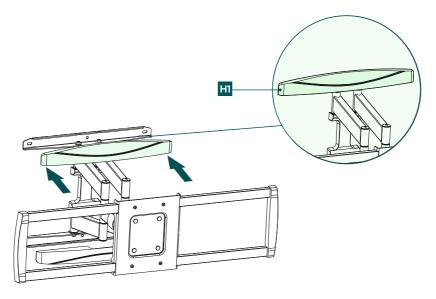
• Then attach the two enclosed covers [H1] to the bracket.
