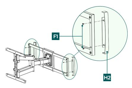
Attach the side covers [H2] using screws [F1] as shown above.
