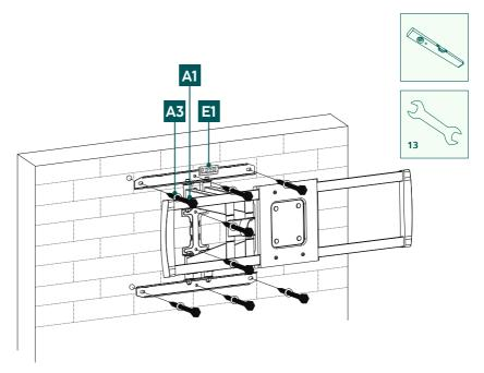
• Attach the wall bracket to the wall as shown above using the enclosed mounting material ([A3] M8 washer, [A1] 8x60 mm screw and the [E1] spirit level).
