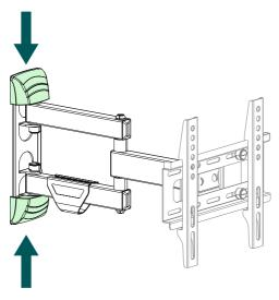
• Then attach the two enclosed covers to the bracket.
