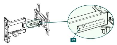
• Then fix the lateral fastening screws using the pipe socket spanner [F2].
