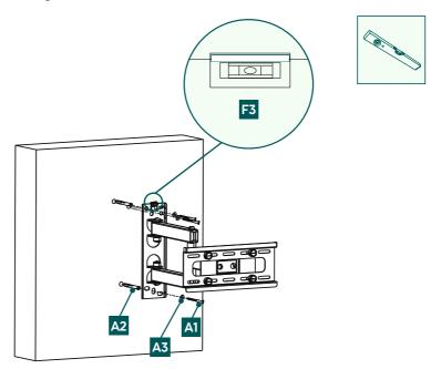
• Attach the wall bracket to the wall as shown above using the enclosed mounting material ([A2] plug, [A3] M8 washer, [A1] 8x60 mm screw and the [F3] spirit level).
