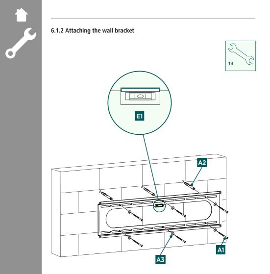
• Attach the wall bracket to the wall as shown above using the enclosed mounting material ([A2] plug, [A3] M8 washer, [A1] 8x60 mm screw and the [E1] spirit level).
