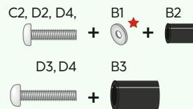
$$\text{M8x50} + \text{Ø 8x5} = \text{M8x45 (D4)}$$
