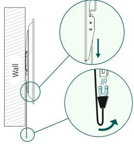
• The ends of the securing cords can be fastened at the back to the wall bracket using the magnets.
