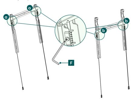
With this wall bracket, you have the option of setting two different heights (a;b). If you do not want to use the pre-mounted setting of the height variant, use the Allen key [F] to release the securing element shown above. Now reattach it at the desired point and re-tighten the securing element using the Allen key [F].
