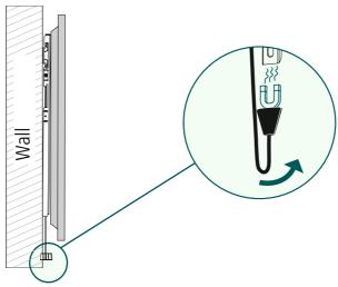
• The ends of the securing cords can be fastened at the back to the wall bracket using the magnets.
