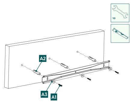
• Attach the wall bracket to the wall as shown above using the enclosed mounting material ([A2] plug, [A3] M8 washer, [A1] 8x60 mm screw and [E] spirit level).
