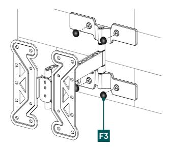
• Then attach the enclosed cover caps [F3] to the hexagon head screws [A1] as shown above.
