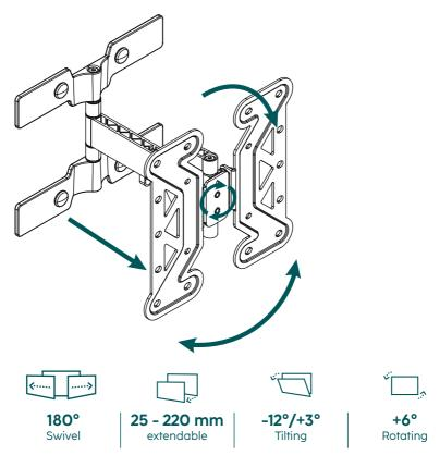
• To adjust the tilt, open the side fastening screws, set the desired tilt and tighten the screws again using the pipe bowl spanner [F1].
