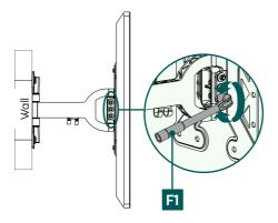
• To adjust the tilt, open the side fastening screws, set the desired tilt and tighten the screws again using the pipe bowl spanner [F1].
