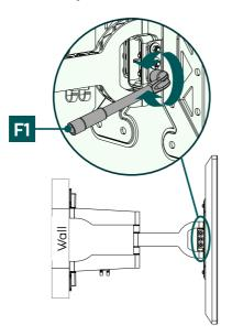
• To adjust the tilt, open the side fastening screws, set the desired tilt and tighten the screws again using the pipe bowl spanner [F1].
