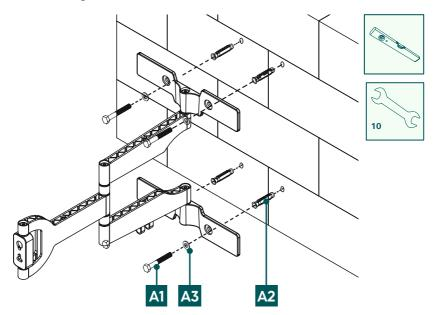
• Attach the wall bracket to the wall as shown above using the enclosed mounting material ([A2] plug, [A3] M8 washer, [A1] 8x60 mm screw and the [F2] spirit level).
