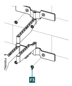
• Then attach the enclosed cover caps [F3] to the hexagon head screws [A1] as shown above.
