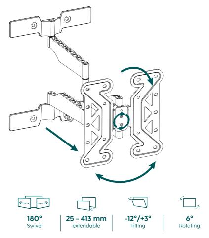
• To adjust the tilt, open the side fastening screws, set the desired tilt and tighten the screws again using the pipe bowl spanner [F1].
