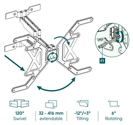
• To adjust the tilt angle, open the fastening screws at the side, set the required tilt and then secure the screws in place again using the enclosed pipe bowl spanner [F1].
