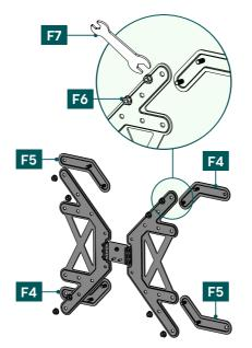
• Mount the supplied adapter plates [F4] / [F5] on the back of the VESA plate using the flange nuts [F6] and spanner [F7].
