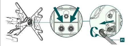
• Loosen the lower flange nuts using the pipe bowl spanner [F1].
