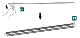
Remove the film from the foam padding [F4] and attach it to the sides of the two VESA arms.
