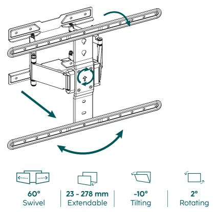
Open the side fastening screws, set the desired tilt and tighten the screws again.
