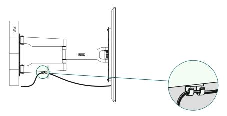
• Stow the cables in the cable holder as shown above.
