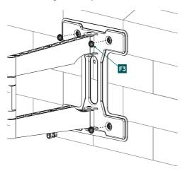
• Then attach the enclosed cover caps [F3] to the hexagon head screws [A1] as shown above.
