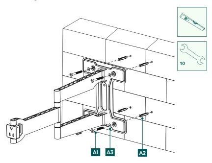
• Attach the wall bracket to the wall as shown above using the enclosed mounting material ([A2] plug, [A3] M8 washer, [A1] 8x60 mm screw and the [F2] spirit level).
