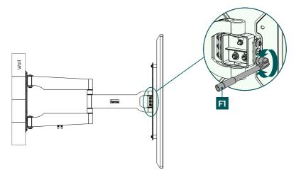
• Then tighten the fixing screws on the side with the enclosed pipe bowl spanner [F1].
