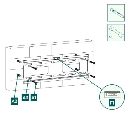
• Attach the wall bracket to the wall as shown above using the enclosed mounting material ([A2] plug, [A3] M8 washer, [A1] 8x60 mm screw and [F1] spirit level).
