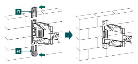
• Attach the two enclosed covers [F1] to the bracket.
