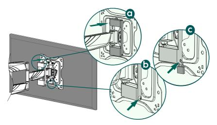
Secure the safety cover on the VESA plate with the enclosed screw (Fig.  $\boldsymbol{b}$ ) or optionally with a padlock (Fig.  $\boldsymbol{c}$ )
