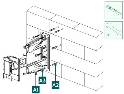
• Attach the wall bracket to the wall as shown above using the enclosed mounting material ([A2] plug, [A3] M8 washer and [A1] 6x55 mm screw).
