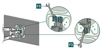
• Secure the fixing screws with the enclosed hexagon ring spanner [F3].
