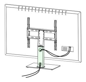
• Use the openings on the mounting pillar for cable management.
