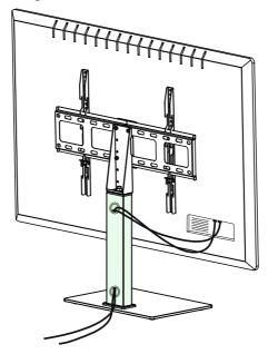
• Use the openings on the mounting pillar for cable management.
