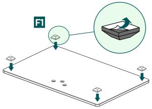
• Attach the self-adhesive rubber feet [F1] to the corners of the base plate as shown above.
