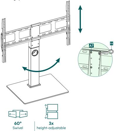
• If the turning function is stiff, loosen the nut [A7] on the joint slightly.
